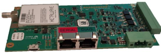
All Xeta9 radios are over-the-air compatible with each other and XetaWave's seamless serial mode allows serial and Ethernet End Points to simultaneously communicate with Ethernet Access Points. The Xeta9s radio also **supports compatibility with MDS TransNET™** master and repeater radios.
