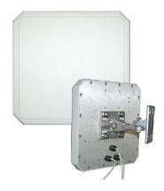
The Laird Connectivity S24517PT is a dual-band, directional sector antenna for use in 802.11n MIMO applications. Enclosed in a low-profile radome, the antenna is mounted using the included articulating mount. The mount can be affixed to a mast or anchored directly to a vertical surface.
